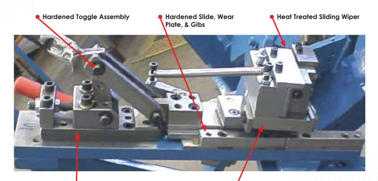
An Adjustable Clevis Assembly is used to control the total amount of slide travel Heat Treated Keeper and Pivot Assembly
