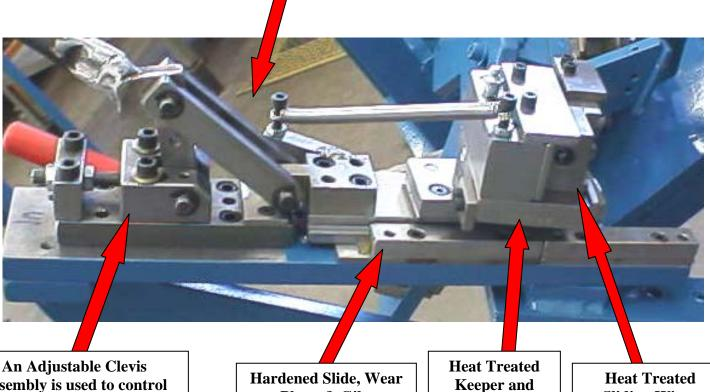
Assembly is used to control the total amount of slide travel
